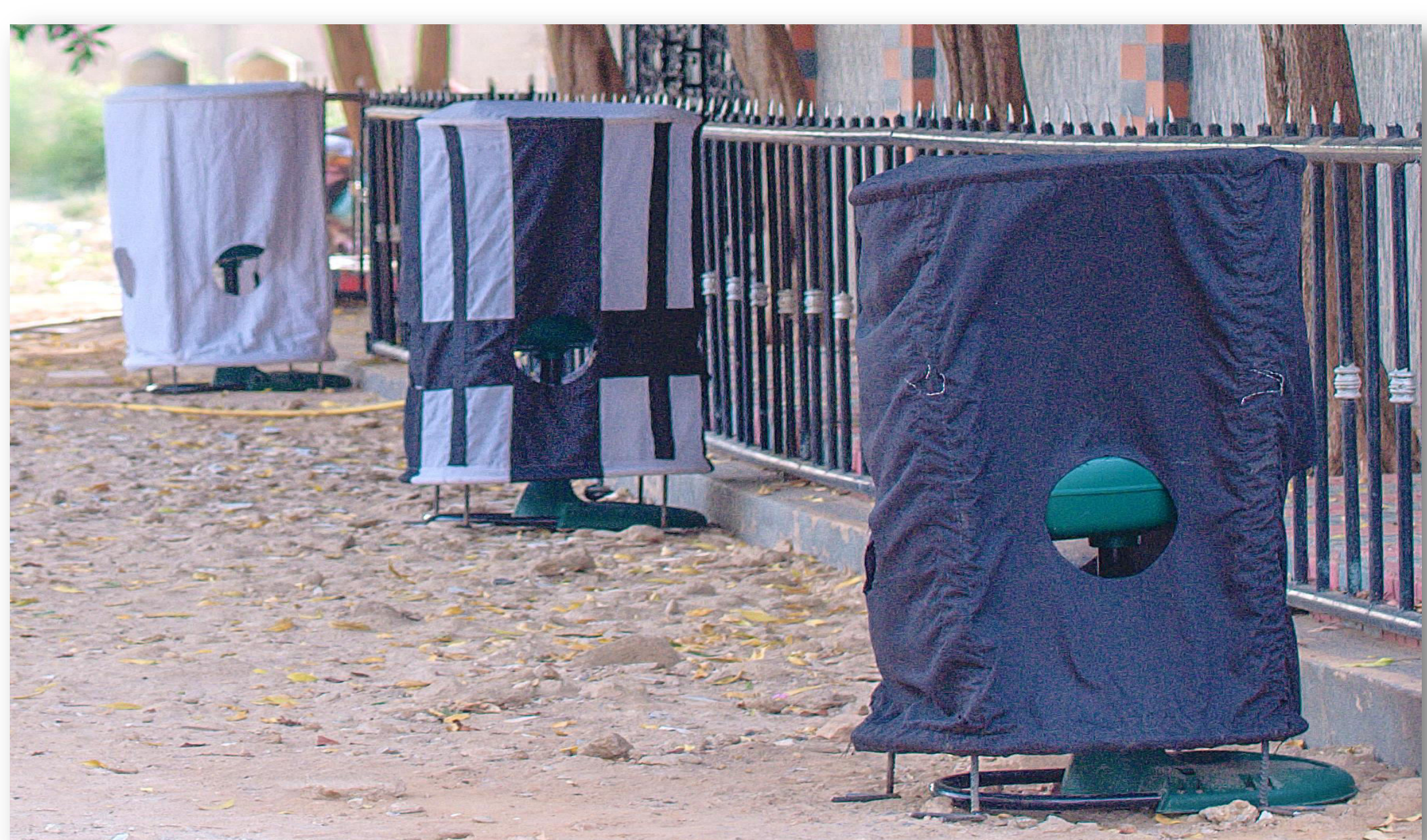
Fig. 2 Experimental setup: MM traps with covers of black, contrasted and white fabric, mosquitoes pass the textile covers from below and the holes in the side, and get sucked into the trap.
